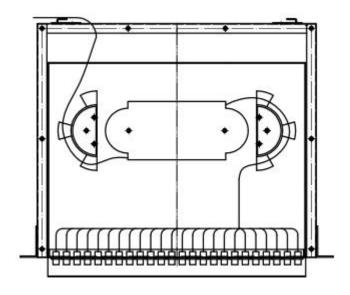
Fiber cable enters into the ODF by split & fix plate at back, and splices with pigtail inside the splice tray after passing through the fiber spool.
